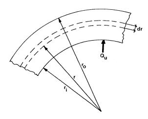
the pressure drop over the annular section from r to r + dr amounts to
